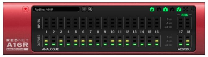
The illustration above shows a RedNet A16R with signal present on all output channels (SRC switched in for AES/EBU channels 17/18). The unit has a single PSU input and a single locked network connection.
