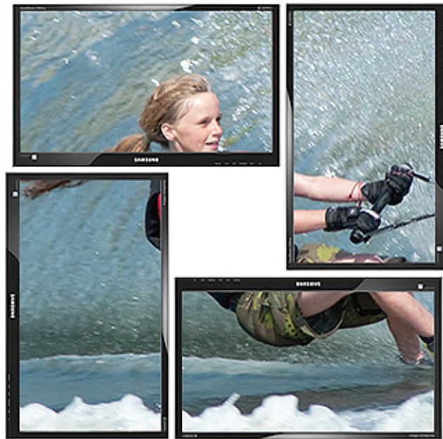
Figure 2-6. Crop the input signal, rotate through 90°, 180°, or 270°; display in landscape and portrait. Arbitrary crop regions can allow the monitors to be artistically arranged, but maintain an undistorted image.
