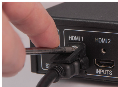
Figure 4-2. Connecting HDMI input cable.
