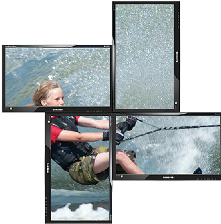
Figure 2-5. Crop the input signal into VideoPlex4000 and display x2 quarters landscape and x2 quarters portrait.
