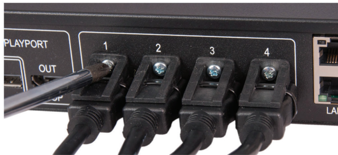
Figure 4-3. Connecting HDMI output cable.
