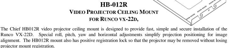
WARNING: IMPROPER INSTALLATION MAY RESULT IN SERIOUS PERSONAL INJURY! All components must be securely fastened to each other and to the ceiling, AND the ceiling MUST be capable of supporting 5 times the total weight of the installation. If it cannot, the ceiling MUST be reinforced.
