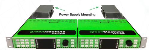
The RFR 6000 shown with two greenMachines installed.
