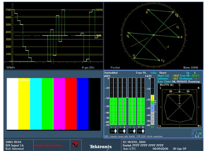
Quad Tile display allows for displays to be viewed simultaneously.
